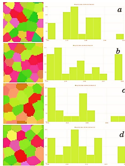
Fig. 12. Microstructure of the model 20-18-16 at 900°C: surface, transverse direction ( a ), surface, longitudinal direction ( b ), centre, transverse direction ( c ), centre, longitudinal direction ( d ).
